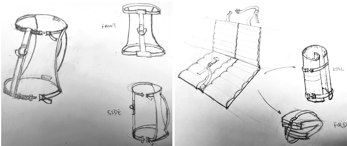
(a) (b) Figure 12. Sketches of our Design Embodiment Beta Prototype depicting (a) the dog harness and (b) the dog seat
